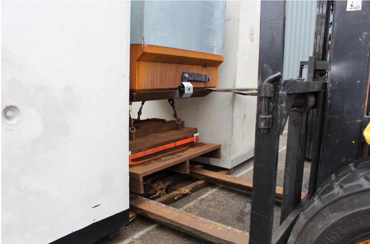
*the test load hangs freely underneath the container*
