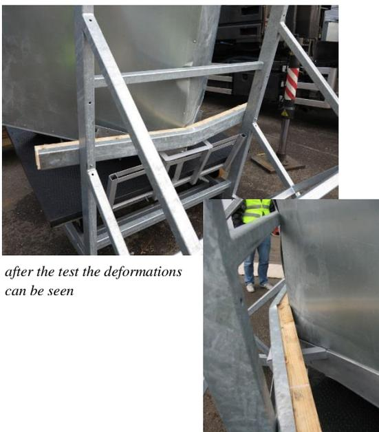
*after the test the deformations can be seen*
