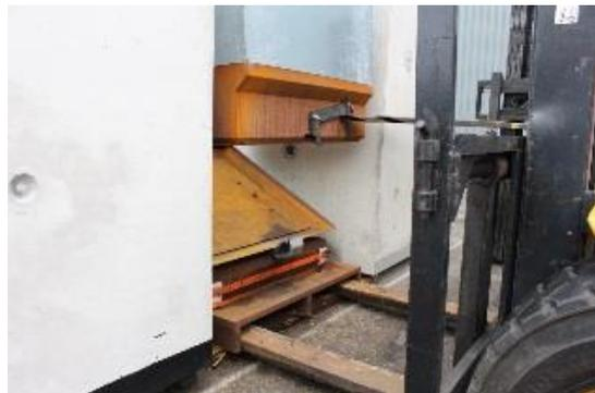
*opening of the bottom hatch containing the test load*
