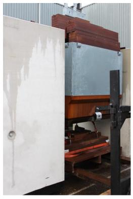
stage 2, 4.000 kg stacked on top of the container, 3.000 kg hangs freely underneath the container
